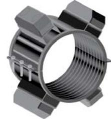
The runners shall be Glass Filled Polymer with ends of the runners beveled to facilitate installation over rough weld beads or the weld ends of misaligned or deformed casing pipe. The runners shall be attached to support structures (risers) at appropriate positions to properly support the carrier pipe within the casing and to ease installation. They shall have a minimum length of 7.0 in. and a minimum width of 2.0 in.
