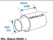
Min. Sleeve Width = Bare Steel Dimension + **50 mm** (2") on each side of the pipe joint.
